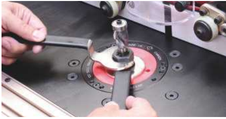
▲ Two spanners are needed for bit swaps but the collet extends well above the table
